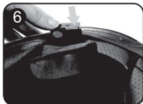
6. With the pin side facing downwards and the charging hole on the left, insert the main unit into the main unit box.
