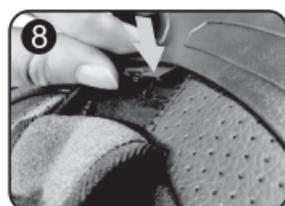
8. After installing the main unit, align the pin of the cover plate with the corresponding empty position in the main unit box and press it in.
