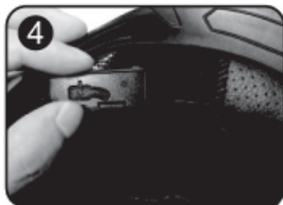
4. Remove the cover plate of the main unit.
